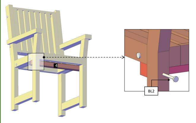
**Step 4:** Use 5/16 x  $3\frac{1}{2}$  bolts (**BL1**) to attach the diagonal supports (**5**) to the seat. After that, use 5/16 x  $4\frac{1}{2}$  (**BL2**) bolts to attach to the legs. Each part has a series of numbers that indicate where to attach the part with the corresponding number.
