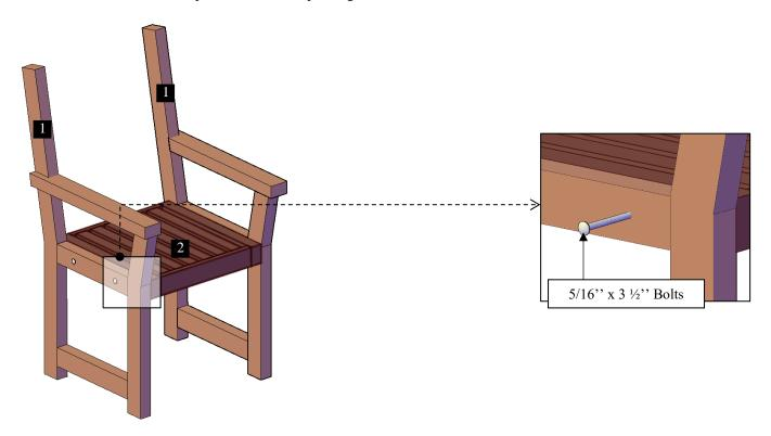
**Step 2:** Attach the backrest (3) to the legs with 5/16" x 3 ½" bolts (a), washers and nuts. Each part has a series of numbers that indicate where to attach the part with the corresponding number.
