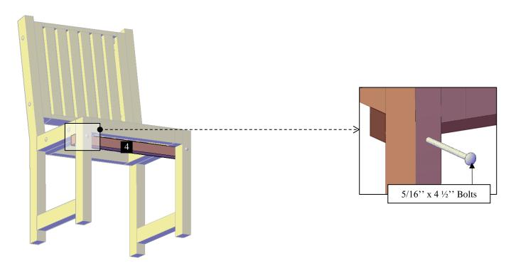
**Step 4:** Finally, use 5/16" x 3 ½" bolts (a) with washers and nuts to attach the diagonal supports (5) to the seat. After that, use 5/16" x 4 ½" bolts (b) with washers and nuts to attach to the legs. Each part has a series of numbers that indicate where to attach the part with the corresponding number.
