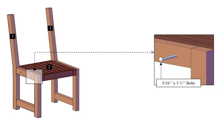
**Step 2:** Attach the backrest (3) to the legs with 5/16" x 3 ½" bolts (a), washers and nuts. Each part has a series of numbers that indicate where to attach the part with the corresponding number.
