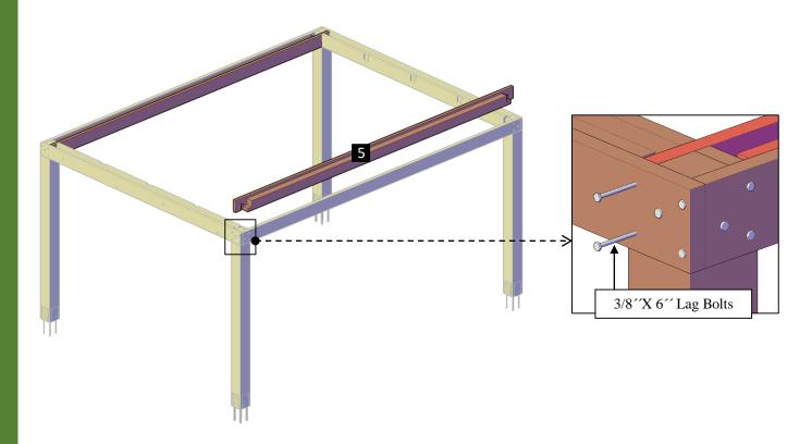
**Step 6:** Attach the long supports with in-between blocking (5) to the long single supports (2) with 3/8" x  $7\frac{1}{4}$ " bolts (E). Each part has a series of numbers that indicate where to attach the part with the corresponding number.
