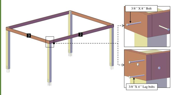
**Step 3:** Put up the short supports with in-between blocking (4), into the post notches as shown and attach to the posts with the single support bolts. After that, attach the short supports with in-between blocking to the short single supports, used 3/8" x 6" lag bolts (**D**) with washers. Each part has a series of numbers that indicate where to attach the part with the corresponding number.
