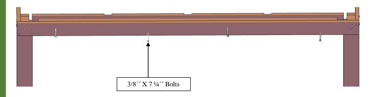
**Step 5:** Put up the long supports with in-between blocking (5), into the post notches as shown and attach to the posts with the single support bolts. After that, attach the long supports with in-between blocking to the long single supports, used 3/8" x 6" lag bolts (**D**) with washers. Each part has a series of numbers that indicate where to attach the part with the corresponding number.
