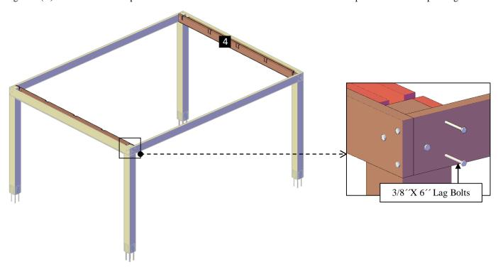
**Step 4:** Attach the shorts supports with in-between blocking (4) to the short single supports (3) with 3/8" x  $7\frac{1}{4}$ " bolts (E). Each part has a series of numbers that indicate where to attach the part with the corresponding number.
