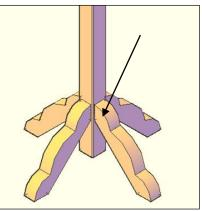
**STEP 2:** Attach the braces to the support, with a Deck screw (2 ½" x #8). Match up the numbers to attach two parts together. Repeat all the process for shorter braces on the top.
