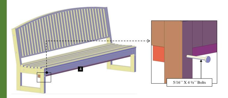
**Step 4:** Finally, use 5/16 'x  $3\frac{1}{2}$  'bolts (**A**) to attach the diagonal supports (**5**) to the seat. After that, use 5/16 'x  $4\frac{1}{2}$  'bolts (**B**) to attach to the legs. Each part has a series of numbers that indicate where to attach the part with the corresponding number.
