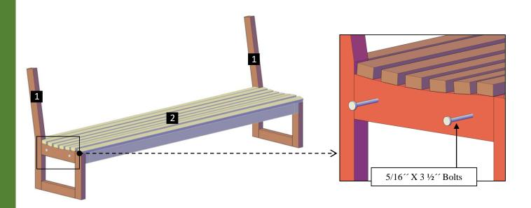
**Step 2:** Attach the backrest (3) to the legs with 5/16 x  $3 \frac{1}{2}$  bolts (A). Each part has a series of numbers that indicate where to attach the part with the corresponding number.
