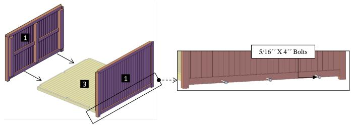
**Step 2:** Use  $5/16^{\prime\prime}$  x  $4^{\prime\prime}$  bolts (**B**) to attach the short fences (**2**) to the floor. After that, attach the short fences to the long fences with  $5/16^{\prime\prime}$  x  $2\frac{1}{2}^{\prime\prime}$  bolts (**A**) and  $3^{\prime\prime}$  deck screws (**c**). Each part has a series of numbers that indicate where to attach the part with the corresponding number.
