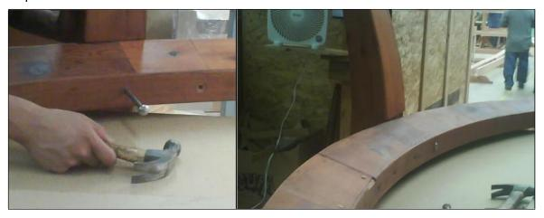
4 Attach part G (joint Connector) to part A & B (arcs), with four bolts, washers & nuts (into four holes marched "6"). Tap the bolt all the way into the wood to set it. Then add a washer and nut and lightly tighten.
