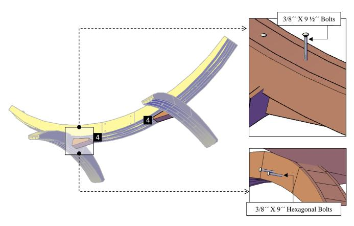
**Step 5:** Attach the support (5) to the arc with 3/8  $\times$  X  $8 \frac{1}{2}$  bolts (F) and with 3/8  $\times$  X 8 bolts (G). Each part has a series of numbers that indicate where to attach the part with the corresponding number. Each part has a series of numbers that indicate where to attach the part with the corresponding number.
