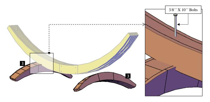
**Step 4:** Attach the knee braces (4) to the arc with 3/8 Y 3/2 bolts (D). Then, use 3/8 Y 3/2 hexagonal bolts (E) to attach the leg to the knee braces (4). Each part has a series of numbers that indicate where to attach the part with the corresponding number.
