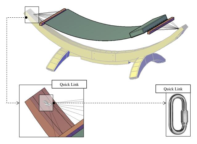
**Step 7:** First attach the eyebolt (**I**) to the arc and hammock bed previously sent. Then place the quick link (**H**) and 1/8" wire cable. Each part has a series of numbers that indicate where to attach the part with the corresponding number.
