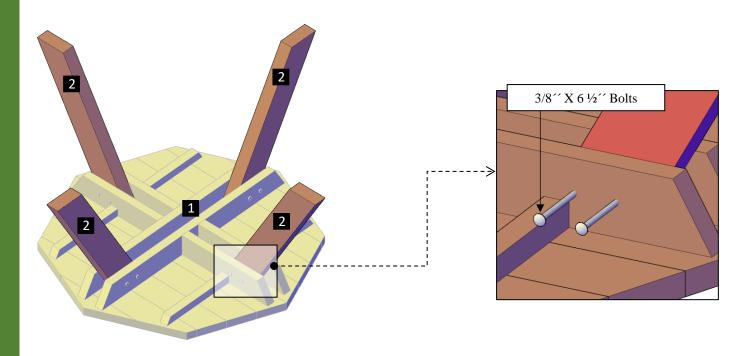
**Step 2:** Use 3/8" x  $6\frac{1}{2}$ " bolts (A) to attach the cross supports (3) to the legs. Each part has a series of numbers that indicate where to attach the part with the corresponding number.
