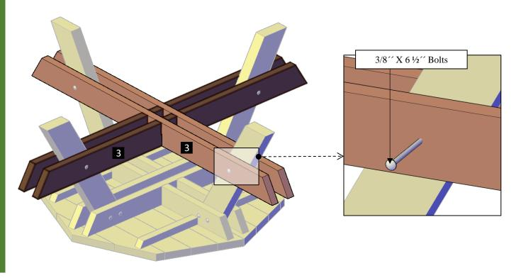
**Step 3:** Turn the table over its feet. After that, attach the benches (5) to the cross supports with 3/8" x 6 ½" bolts (A). Each part has a series of numbers that indicate where to attach the part with the corresponding number.
