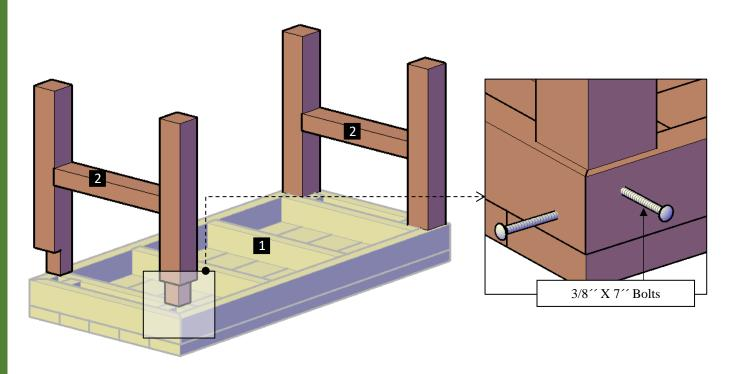
**Step 2:** Attach the shelf (3) to the legs with 3/8 ' X 6' bolts (B). Each part has a series of numbers that indicate where to attach the part with the corresponding number.
