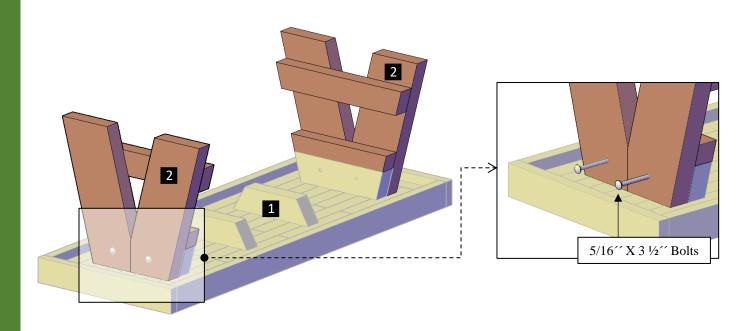
**Step 2:** Finally, attach the diagonal supports (3) to the legs and to the seat with  $5/16^{\prime\prime}$  x  $3\frac{1}{2}^{\prime\prime}$  bolts (A), washers (B) & nuts (C). Each part has a series of numbers that indicate where to attach the part with the corresponding number.
