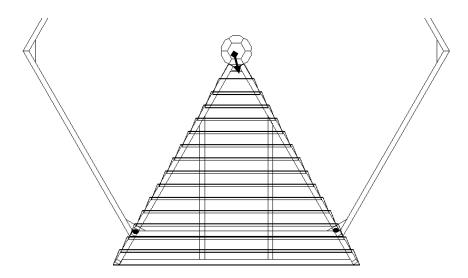
Attach the panels between them with lag bolts, washers and nuts.
