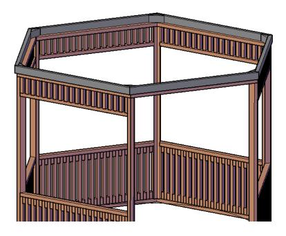
**STEP 5:** Attach the Roof panel to roof base and center piece with bolts, washers & nuts. (Match up the numbers to attach the two parts together). Tap the bolt all the way into the wood to set it. Then add a washer and nut and lightly tighten.
