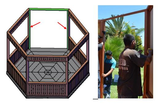
**STEP 4:** Attach the timbers together to form the base of the roof with bolts (3 ½" x 5/16)), washers & nuts. (Match up the numbers to attach the two parts together). Tap the bolt all the way into the wood to set it. Then add a washer and nut and lightly tighten.
