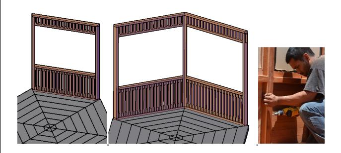
**STEP 3:** Attach the door frame to the wall panels with deck screws  $3" \times #8$ .
