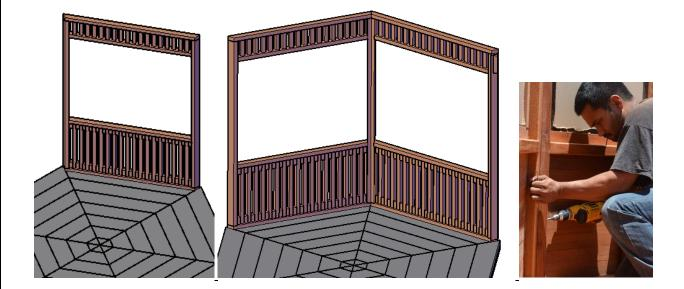
**STEP 3:** Attach the door frame to the wall panels with deck screws 3" x #8.
