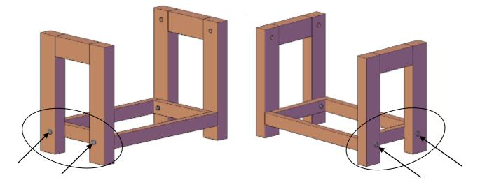
**Step 2:** Attach the top to both legs with 2 carriage bolts, washers and nuts each. Make sure that the numbers written next to the predrilled holes match.
