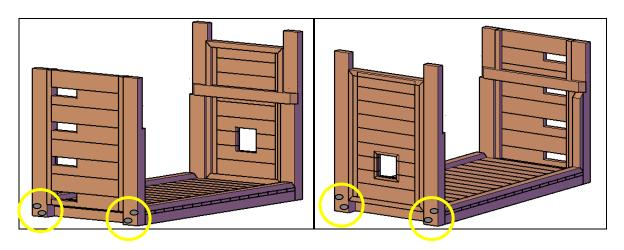
**STEP 2:** Attach back wall to side wall & climbing ladder, with two bolts ( $4 \frac{1}{2}$ " x 5/16"), washers & nuts per side. Tap the bolt all the way into the wood to set it. Then add a washer and nut and lightly tighten.
