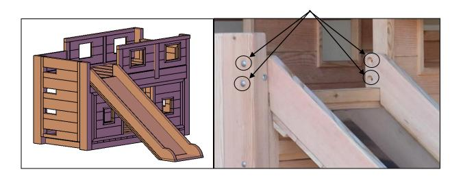
**STEP 5:** Attach both sides of roof to front & back walls, with two bolts per side (3"x 5 1/6"), washers & nuts (into holes marked). Tap the bolt all the way into the wood to set it. Then add a washer and nut and lightly tighten.
