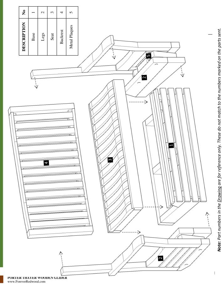
**Step 1:** First adjust the metal plaques (4) to the legs (2) on the outer sides with 3/8" bolts (A). Place a 5/16" nuts (B) in front and back of the metal plaque to tighten it. Each part has a series of numbers that indicate where to attach the part with the corresponding number
