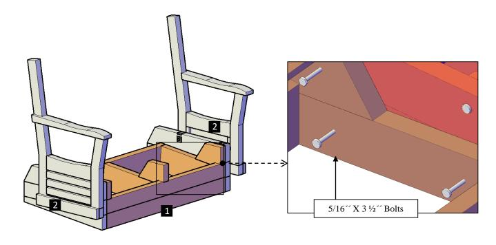
**Step 3:** Attach the seat (3) to the legs with  $5/16^{\prime\prime}$  x  $3\frac{1}{2}^{\prime\prime}$  bolts (A), as shown below. Each part has a series of numbers that indicate where to attach the part with the corresponding number.
