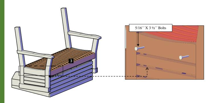
**Step 4:** Finally, use 5/16 'x  $3\frac{1}{2}$ ' bolts (A) to attach the backrest (4) to the legs. Each part has a series of numbers that indicate where to attach the part with the corresponding number.
