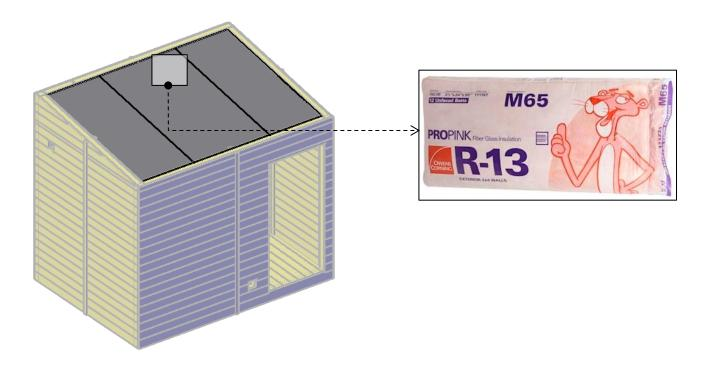
Step 18: Place the roof boards that were removed from the roof panels (13) with 2" deck screws (DS2).
