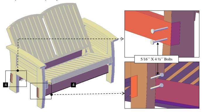
**Step 4:** Finally, attach the diagonal supports (5) to the supports with 5/16" x 3  $\frac{1}{2}$ " bolts (A) and to the legs with 5/16" x 4" bolts (C). Each part has a series of numbers that indicate where to attach the part with the corresponding /number.
