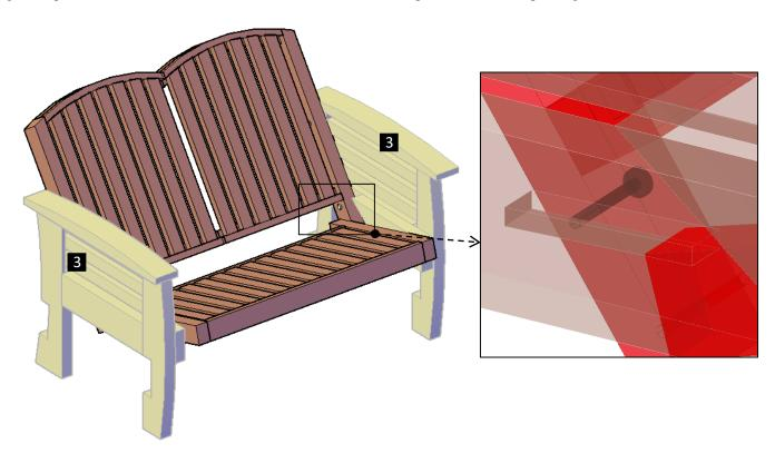
**Step 3:** Attach the supports **(4)** to the legs with 5/16 x  $4\frac{1}{2}$  bolts **(B)**. Each part has a series of numbers that indicate where to attach the part with the corresponding number.
