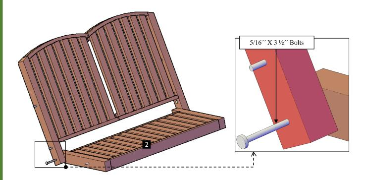
**Step 2:** Insert the seat and backrest bolts into the predrilled cut outs on the legs (3). Attach one leg first, after that, attach the other leg. Each part has a series of numbers that indicate where to attach the part with the corresponding number.
