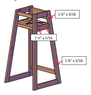
**Step 4.** Attach front support and leg to seat with 4 carriage bolts (1  $\frac{3}{4}$ " x 5/16), washers and nuts. Match the numbers next to the predrilled holes on the pieces. Tap the carriage bolts all the way into the wood, then attach the washers, nuts and tighten with  $\frac{1}{2}$ -inch ratchet. Do not over-tighten.
