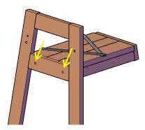
**Step 2.** Attach backrest to leg with 2 carriage bolts (1  $\frac{3}{4}$ " x 5/16), washers and nuts. Match the numbers next to the predrilled holes on the backrest to the numbers on the chair side. Tap the carriage bolts all the way into the wood, then attach the washers, nuts and tighten with  $\frac{1}{2}$ -inch ratchet. Do not over-tighten.
