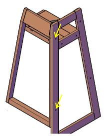
**Step 3.** Attach backrest and leg to seat with 4 carriage bolts, washers and nuts. Match the numbers next to the predrilled holes on the pieces. Tap the carriage bolts all the way into the wood, then attach the washers, nuts and tighten with ½-inch ratchet. Do not over-tighten.
