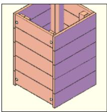
**STEP 2:** Attach wall to floor, with two bolts 2 ½" x 5/16", washers & nuts. Tap the bolt all the way into the wood to set it. Then add a washer and nut and lightly tighten. *Repeat this step for the other side*
