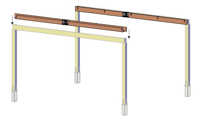
**Step 4:** Use 3/8" x 12" lag bolts (**LB2**) to attach the single supports-B (**3**) to the posts and use 3/8" x 4" lag bolts (**LB3**) to attach the supports together. Check the marked on each support and place as drawings shown.
