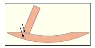
**STEP 2:** Attach rear legs to seat with two bolts  $4^{n}x 5/16^{n}$ , washers & nuts. Repeat this step to attach the other sides
