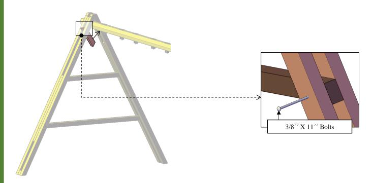
**Step 9:** Pull out the second cross supports and line up to match the predrilled hole. After that, use 3/8" X 11" Bolts (A) with washer and nut to attach.
