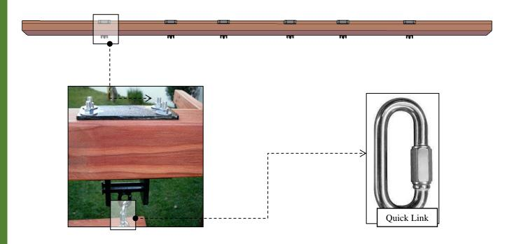
**Step 7:** Attach the main structural timber (3) to the frames legs with 3/8" X 12" bolts (C) with washer and nut. Each part has a series of numbers that indicate where to attach the part with the corresponding number.
