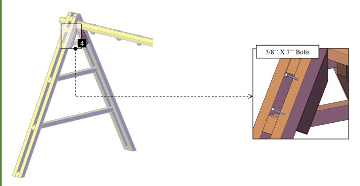
**Step 11:** Attach the knee braces (5) to the main structural timber with 3/8" x 10" bolts (**E**) and to the frame legs with 3/8" x 7" bolts (**D**). Don't forget washers and nuts. Each part has a series of numbers that indicate where to attach the part with the corresponding number.
