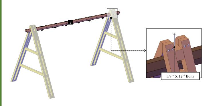
**Step 8:** Pull out the first cross supports and line up to match the predrilled hole. After that, use 3/8 "X 11" Bolts (**A**) with washer and nut to attach.
