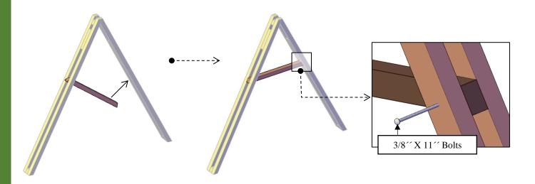
**Step 3:** Use 3/8" X 11" Bolts (**A**) with washer and nut to attach the lower main support (**2**) to the frame legs. Each part has a series of numbers that indicate where to attach the part with the corresponding number.
