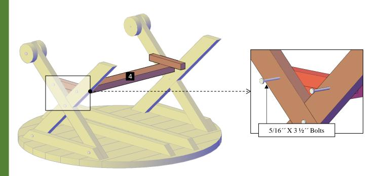
**Step 4:** Use 5/16" x  $3\frac{1}{2}$ " bolts (**A**) to attach the diagonal supports (**5**) to the tabletop and to the legs. Each part has a series of numbers that indicate where to attach the part with the corresponding number
