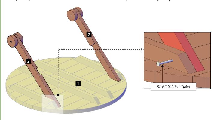
Step 2: Attach the other legs (3) to the tabletop with 5/16" x 3 ½" bolts (A). The legs will be attached together with 5/16" x 2" bolts (B). Each part has a series of numbers that indicate where to attach the part with the corresponding number.
