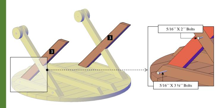
**Step 3:** Attach the support (4) to the legs with 5/16" x 3 ½" bolts (A). Each part has a series of numbers that indicate where to attach the part with the corresponding number.
