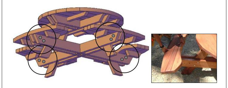
**Step 6:** The final step is to attach diagonal supports at 45 degree angles underneath the benches. Match up the numbers on the diagonal support ends to the numbers written underneath the benches and table's leg. Attach with 2 screws to bench and 2 screws to leg. Repeat this step to attach all the other diagonal supports.
