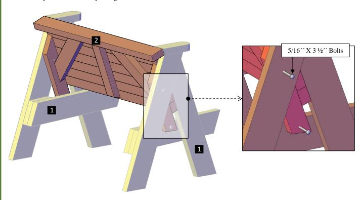
**Step 2:** Finally, use  $5/16^{\prime\prime}$  x  $3\frac{1}{2}^{\prime\prime}$  bolts (A) and  $5/16^{\prime\prime}$  x  $5^{\prime\prime}$  bolts () to attach the legs to the seat (3). Each part has a series of numbers that indicate where to attach the part with the corresponding number.
