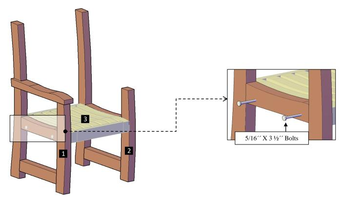
**Step 2:** Attach the backrest (4) to the legs with 5/16 ′′ x  $3 \frac{1}{2}$  ′′ bolts (A). Each part has a series of numbers that indicate where to attach the part with the corresponding number.
