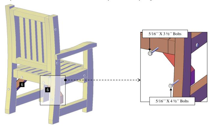
**Step 5:** Use 5/16" x 4 ½" bolts (**B**) to attach the support (**7**) to the legs. Each part has a series of numbers that indicate where to attach the part with the corresponding number.
