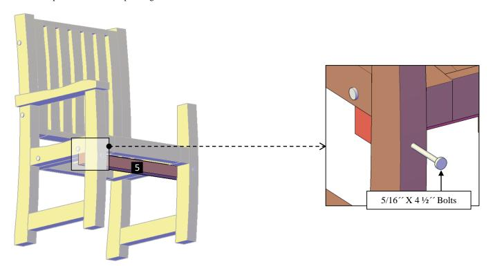
**Step 4:** Attach the diagonal supports (6) to each seat with 5/16" x 3  $\frac{1}{2}$ " bolts (A) and to the legs with 5/16" x 4  $\frac{1}{2}$ " bolts (B). Each part has a series of numbers that indicate where to attach the part with the corresponding number.
