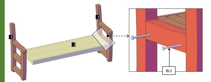
**Step 2:** Attach the backrest (3) to the legs with  $5/16^{\prime\prime} \times 4 \frac{1}{2^{\prime\prime}}$  bolts (**BL1**). Each part has a series of numbers that indicate where toattach the part with the corresponding number.
