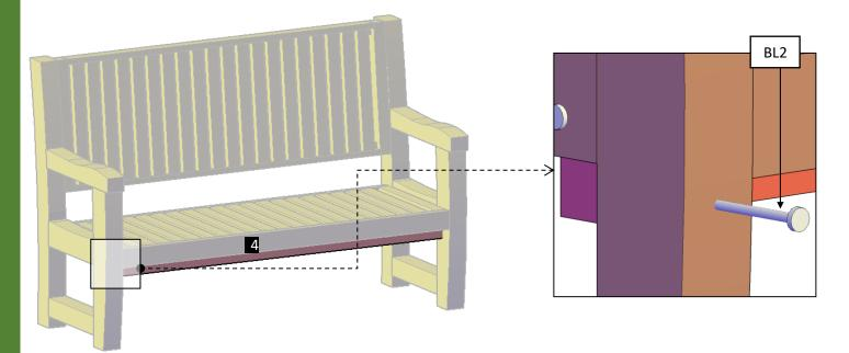
**Step 4:** Use 5/16 x  $3\frac{1}{2}$  bolts (**BL3**) to attach the diagonal supports (**5**) to the seat. After that, use 5/16 x  $5\frac{1}{2}$  bolts (**BL2**) bolts to attach the legs. Each part has a series of numbers that indicate where to attach the part with the corresponding number.
