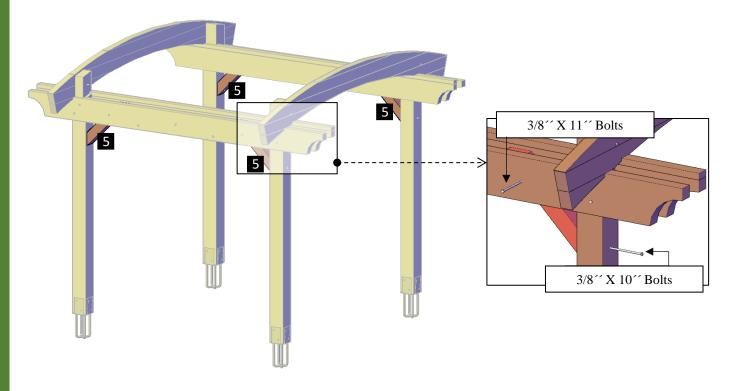
**Step 7:** Attach the secondary knee braces (6) to the posts with 3/8 x 10 bolts (E) and to the arched rafters with 3/8 x 8 bolts (F). Each part has a series of numbers that indicate where to attach the part with the corresponding number.
