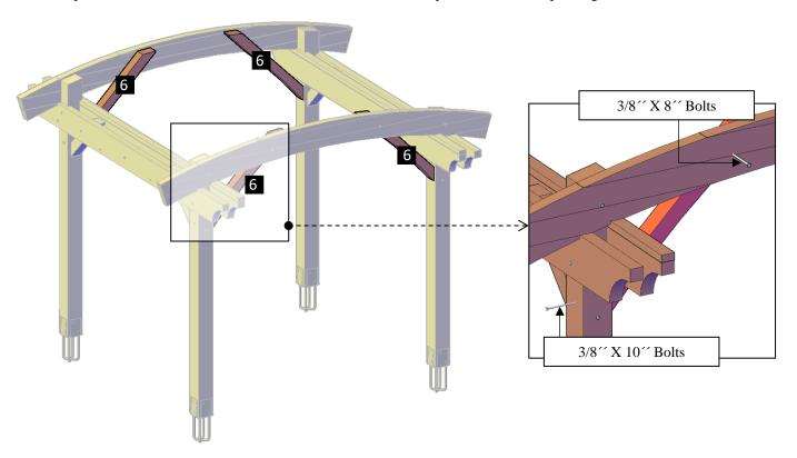
**Step 8:** Use 8" x 3" deck screws (**D**) to attach the central arched rafters (**7**) to the supports. Each part has a series of numbers that indicate where to attach the part with the corresponding number.
