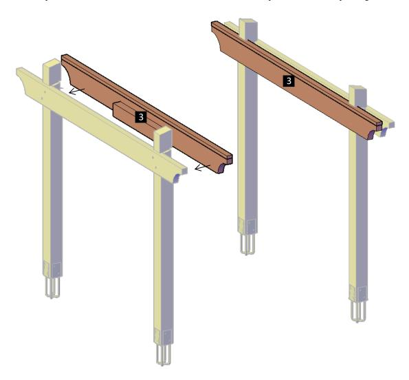
**Step 4:** Attach the single supports (2) to the supports with in-between blocking (3), use 3/8" X 11" bolts (B). The quantity of bolts depends on the length of the supports.
