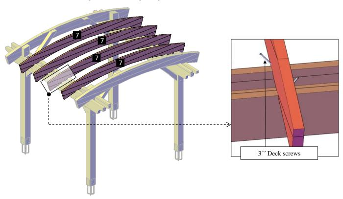
**Step 9:** Use 8" x 3" deck screws (**D**) to attach the Slats-A (**8**) and the Slats-B (**9**) to the arched rafters. Each part has a series of numbers that indicate where to attach the part with the corresponding number.
