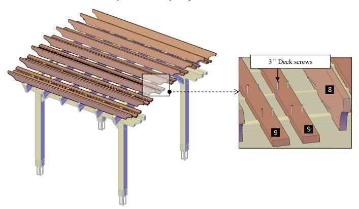
Step 10: Finally, attach the boots (10) to the posts with 8" x 3" deck screws (D).
