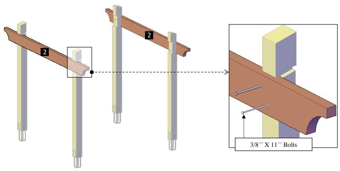
**Step 3:** Place the supports with in-between blocking (3), into the post notches as shown and attach to the post with the single support bolts. Each part has a series of numbers that indicate where to attach the part with the corresponding number.
