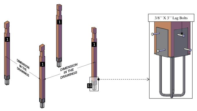
**Step 2:** Attach the single supports (2) to the posts with 3/8  $\times$  X 11  $\times$  bolts (B). Each part has a series of numbers that indicate where to attach the part with the corresponding number.
