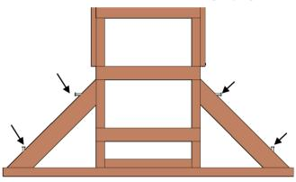
**Step 3:** Attach the support to the ladders, with four bolts (3 ½" x 5/16"), washers & nuts. (Match up the numbers to attach the two parts together) Tap the bolt all the way into the wood to set it. Then add a washer and nut and lightly tighten.
