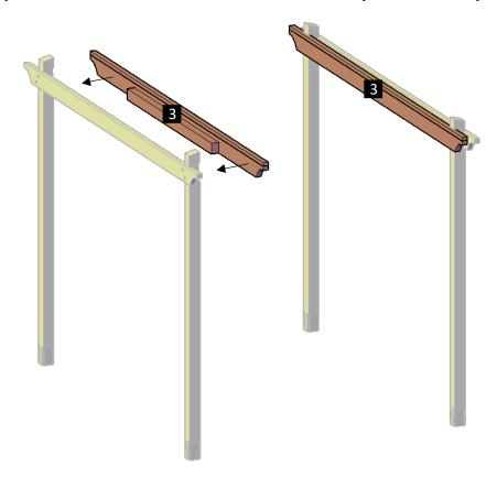
**Step 4:** Attach the single supports (2) to the supports with in-between blocking (3), use 3/8 'x 6' bolts (C). The quantity of bolts depends on the length of the supports.
