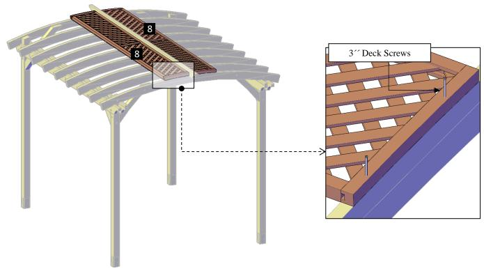
**Step 10.2:** Attach the slats (8) to the arched rafters with  $8^{\prime\prime} \times 3^{\prime\prime}$  deck screw (**D**). Each part has a series of numbers that indicate where to attach the part with the corresponding number.
