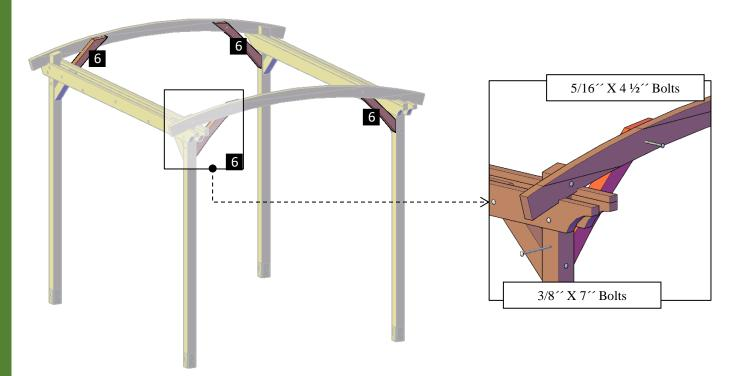
**Step 8:** Use  $8^{\prime\prime} \times 3^{\prime\prime}$  deck screws (E) to attach the rest of arched rafters (4) to the supports. Each part has a series of numbers that indicate where to attach the part with the corresponding number.
