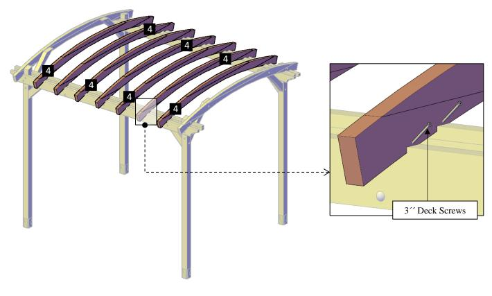
**Step 9:** Attach the central slat (7) to the arched rafters with  $8^{\prime\prime} \times 3^{\prime\prime}$  deck screws (**D**). Each part has a series of numbers that indicate where to attach the part with the corresponding number.
