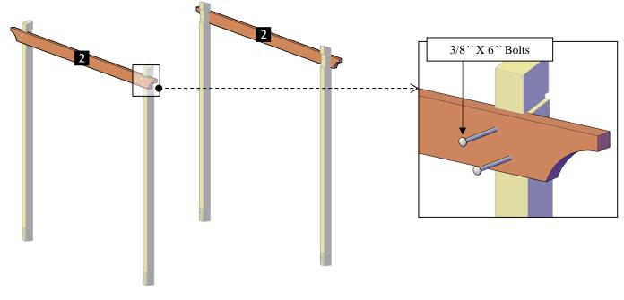
**Step 3:** Put up the supports with in-between blocking (3), into the post notches as shown and attach to the posts with the single support bolts. Each part has a series of numbers that indicate where to attach the part with the corresponding number.
