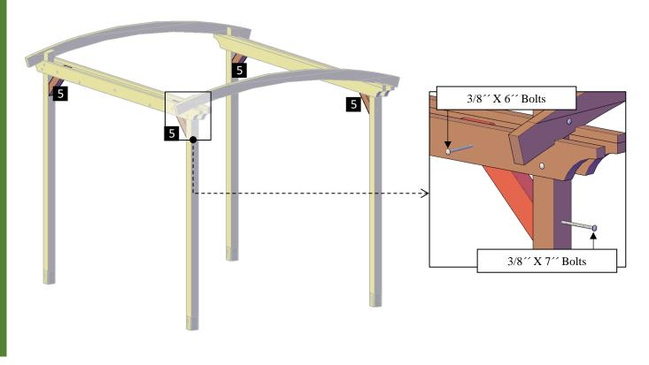
SMALL ARCHED PERGOLA KITS www.ForeverRedwood.com **Step 7:** Attach the secondary knee braces (6) to the arched rafters with  $5/16^{\prime\prime} \ge 4\frac{1}{2}^{\prime\prime}$  bolts (G) and to the posts with  $3/8^{\prime\prime} \ge 7^{\prime\prime}$  bolts (F). Each part has a series of numbers that indicate where to attach the part with the corresponding number.
