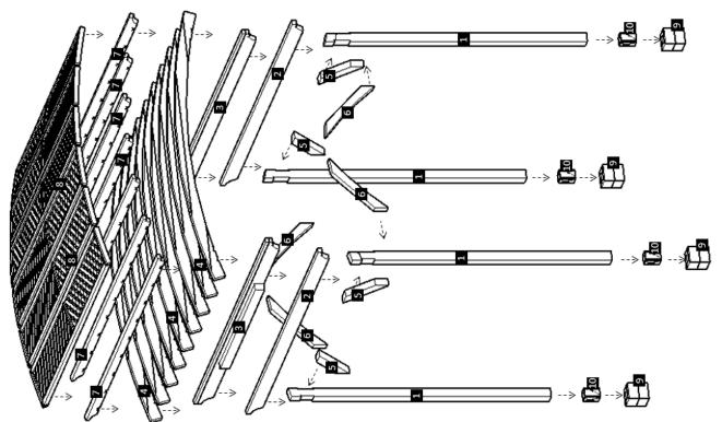
SMALL ARCHED PERGOLA KITS www.ForeverRedwood.com **NOTE:** In order to know where the post needs to be placed, check the numbers on them. If the post is not marked, then place the single Supports on the ground to locate the markings for each post position and clearly set your bearings. ("Don't attach yet, only place them on the ground to begin with").
