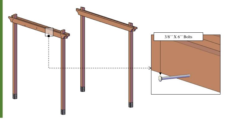
SMALL ARCHED PERGOLA KITS www.ForeverRedwood.com **Step 5:** Attach the perimeter arched rafters (4) to the posts with 3/8 x 5 bolts (**D**) and to the supports with 8 x 3 deck screws (**E**). Each part has a series of numbers that indicate where to attach the part with the corresponding number.
