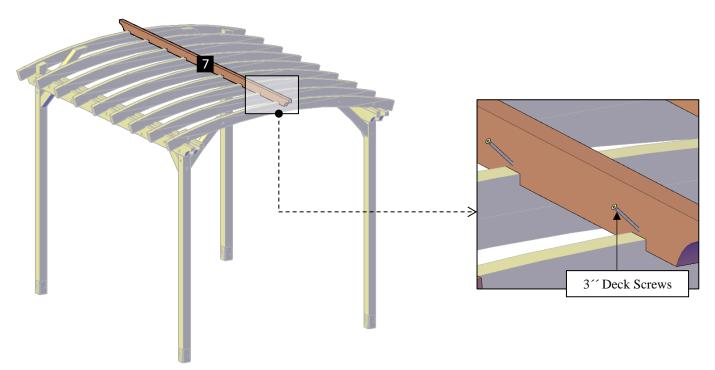
Step 10: Continue attaching the slats (8) and the roof lattice panels (7) to the arched rafters.
