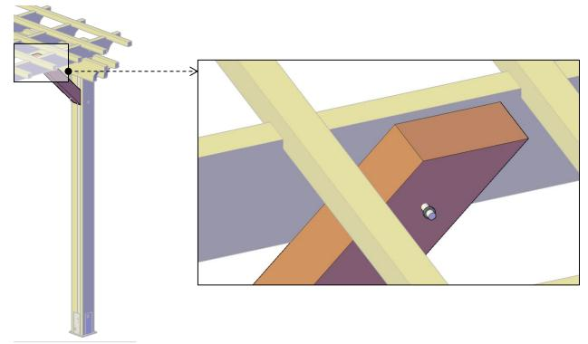
Step 3: The bolt of the post and the knee brace must be flush with the post.
