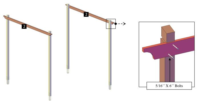
**Step 3:** Put up the supports with in-between blocking (3), into the post notches as shown and attach to the posts with the single support bolts. Each part has a series of numbers that indicate where to attach the part with the corresponding number.
