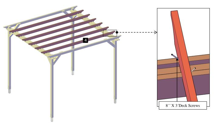
**Step 9:** Use 8" x 3" deck screws (**E**) to attach each slats (**7**) to the rafters. Each part has a series of numbers that indicate where to attach the part with the corresponding number.
