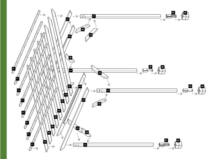
**NOTE:** In order to know where the post needs to be placed, check the numbers on them. If the post is not marked, then place the single Supports on the ground to locate the markings for each post position and clearly set your bearings. ("Don't attach yet, only place them on the ground to begin with").
