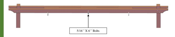
**Step 5:** Attach the perimeter rafters first (4) to the posts with 5/16 'x 5' bolts (**D**) and to the supports with 8' x 3' deck screws (**E**). Each part has a series of numbers that indicate where to attach the part with the corresponding number.
