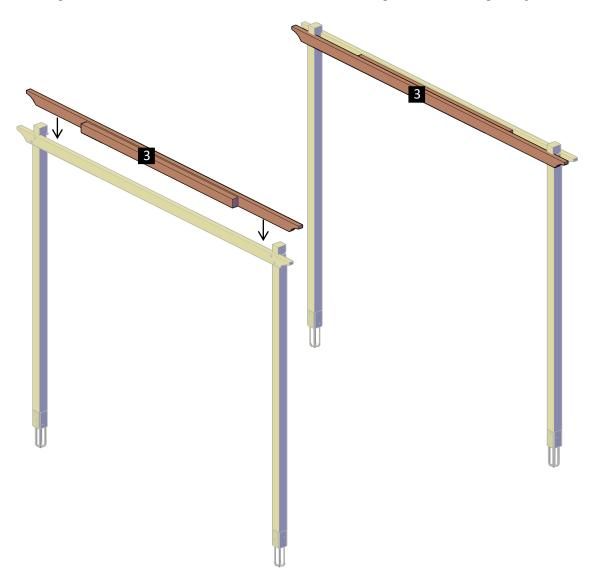
**Step 4:** Attach the single supports (2) to the supports with in-between blocking (3), use 5/16 x 6 bolts (C). The quantity of bolts depends on the length of the supports.
