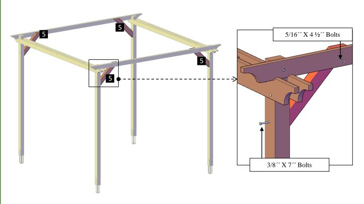
**Step 7:** Attach the main knee braces (6) to the posts with 3/8 ' x 7'' bolts (F) and to the supports with 5/16 ' x 6'' bolts (C). Each part has a series of numbers that indicate where to attach the part with the corresponding number.
