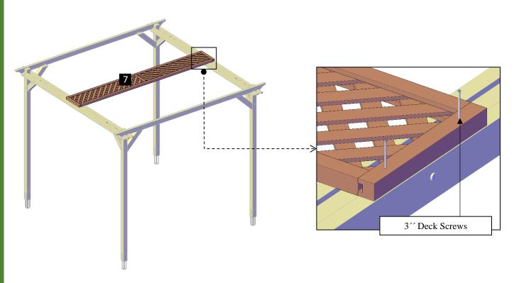
**Step 9:** Use 8" x 3" deck screws (**E**) to attach the rafters (**4**) to the supports. Each part has a series of numbers that indicate where to attach the part with the corresponding number.
