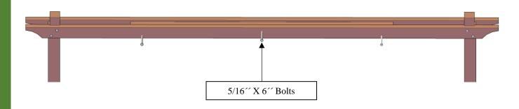
**Step 5:** Attach the perimeter rafters first (4) to the posts with  $5/16^{\prime\prime}$  x  $5^{\prime\prime}$  bolts (**D**) and to the supports with  $8^{\prime\prime}$  x  $3^{\prime\prime}$  deck screws (**E**). Each part has a series of numbers that indicate where to attach the part with the corresponding number.
