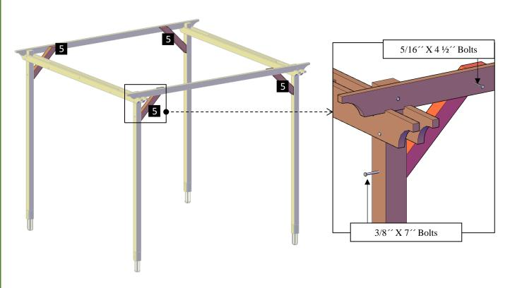
**Step 7:** Attach the main knee braces (6) to the posts with 3/8" x 7" bolts (F) and to the supports with 5/16" x 6" bolts (C). Each part has a series of numbers that indicate where to attach the part with the corresponding number.
