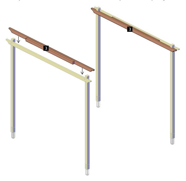
**Step 4:** Attach the single supports (2) to the supports with in-between blocking (3), use 5/16 'x 6 'bolts (C). The quantity of bolts depends on the length of the supports.
