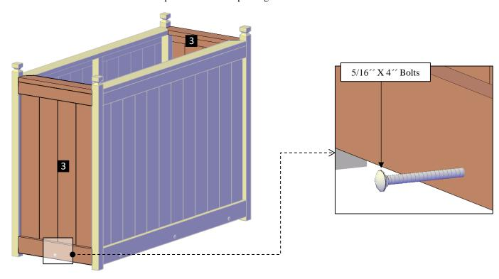
**Step 3:** Attach the short fences (3) to the long fences with 5/16" x 3" bolts (B) with washers and nuts. After that, use 3" deck screws (C).
