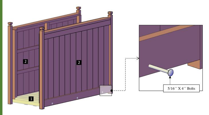
**Step 2:** Use 5/16" x 4" bolts (**A**) with washers and nuts to attach the short fences (**3**) to the floor. Each part has a series of numbers that indicate where to attach the part with the corresponding number.
