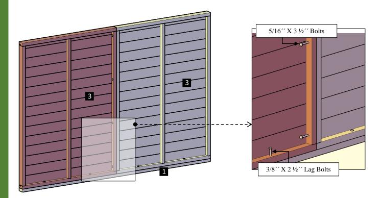
Repeat this step to assemble the lateral walls.
