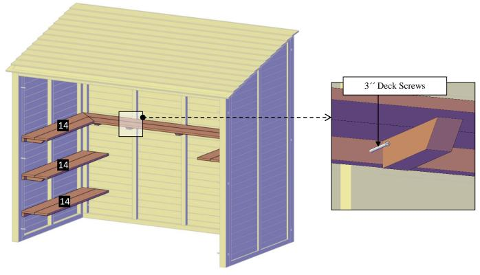
**Step 13:** Finally, use 3" Deck Screws (I) to attach the knee braces (15) to the shelves and to the walls. Each part has a series of numbers that indicate where to attach the part with the corresponding number.
