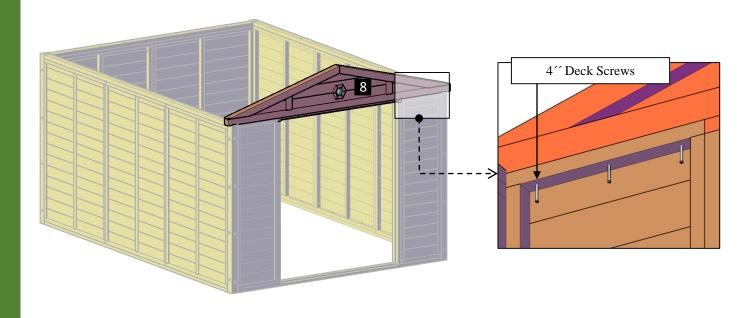
**Step 6:** Attach the central triangles (9) to the lateral walls with 4" deck screws (**D**). Each part has a series of numbers that indicate where to attach the part with the corresponding number.
