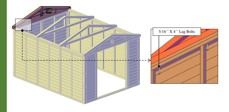
**Step 8:** Attach the roof panels (11) to the perimeter triangles with 5/16" x 5" bolts (C). After that, use 3/8" x 7" bolts (F) to attach to the central triangles. Finally, put <u>Exterior Clear Silicone</u> on the roof panels joints. Each part has a series of numbers that indicate where to attach the part with the corresponding number.
