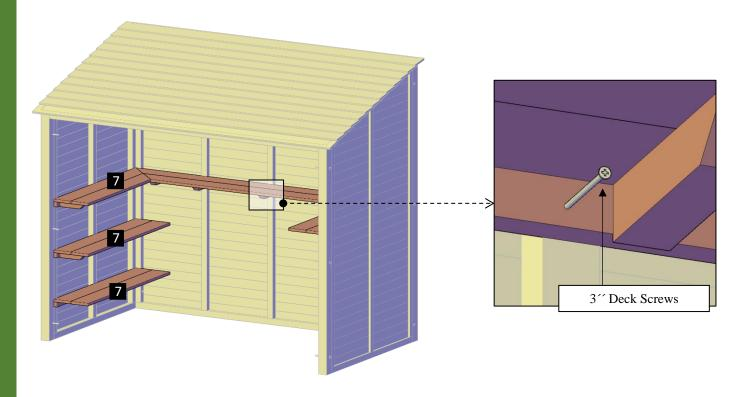
**Step 8:** Finally, use 3" Deck Screws (**D**) to attach the knee braces (**8**) to the shelves and to the walls. Each part has a series of numbers that indicate where to attach the part with the corresponding number.
