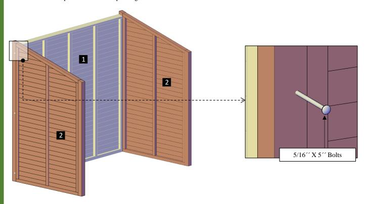
**Step 2:** Attach the frontal wall (3) to the lateral walls with 5/16 x 5 bolts (A). Each part has a series of numbers that indicate where to attach the part with the corresponding number.
