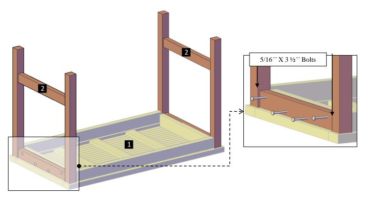
**Step 2:** Attach the support (3) to the legs with 5/16'' x 3 ½'' bolts (A). Each part has a series of numbers that indicate where to attach the part with the corresponding number.
