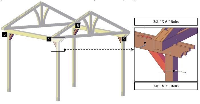
**Step 9:** Attach the secondary knee braces (6) to the triangles with 3/8" x 6" Bolts (C) and to the posts with 3/8" x 7" bolts (E). Each part has a series of numbers that indicate where to attach the part with the corresponding number.
