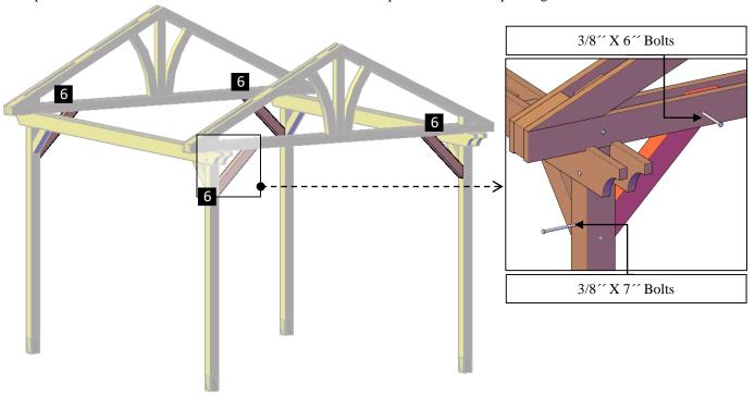
**Step 10:** Use 3" deck screws (**D**) to attach the central triangle (**4**) to the supports. Each part has a series of numbers that indicate where to attach the part with the corresponding number.
