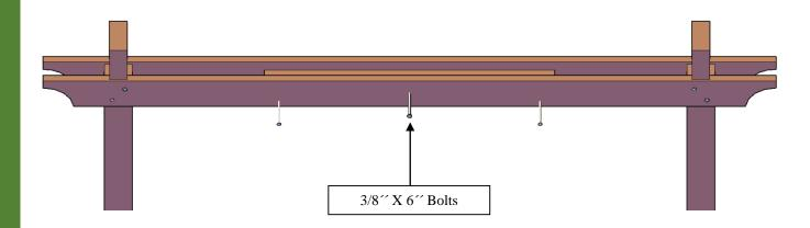
**Step 5:** Attach the triangles (4) to the posts with 3/8" x 6" bolts (C) and to the supports with 3" deck screws (D). Each part has a series of numbers that indicate where to attach the part with the corresponding number.
