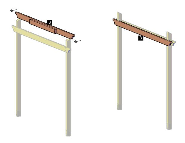
**Step 4:** Attach the single supports to the supports with in-between blocking, use 3/8 ' X 6' bolts (C). The quantity of bolts depends on the length of the supports.
