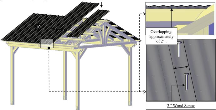
**Step 14:** Use 2" Wood Screw with Neoprene Washer to attach the ridge cap (18). Each part has a series of numbers that indicate where to attach the part with the corresponding number.
