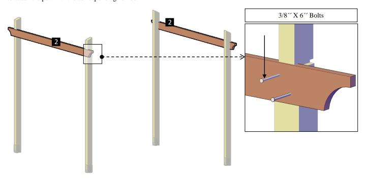
**Step 3:** Put up the supports with in-between blocking (3), into the post notches as shown and attach to the posts with the single support bolts. Each part has a series of numbers that indicate where to attach the part with the corresponding number.
