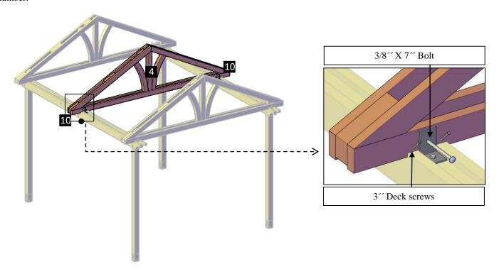
**Step 8:** Attach the main knee braces (5) to the supports with 3/8" x 6" Bolts (C) and to the posts with 3/8" x 7" bolts (E). Each part has a series of numbers that indicate where to attach the part with the corresponding number.
