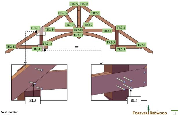
Step 17: Use 3/8" x 9 <sup>1</sup>/<sub>4</sub>" bolts (BL6) to attach the roof trusses (1) to the perimeter posts. Check the marked on each roof truss and place as drawings shown.
