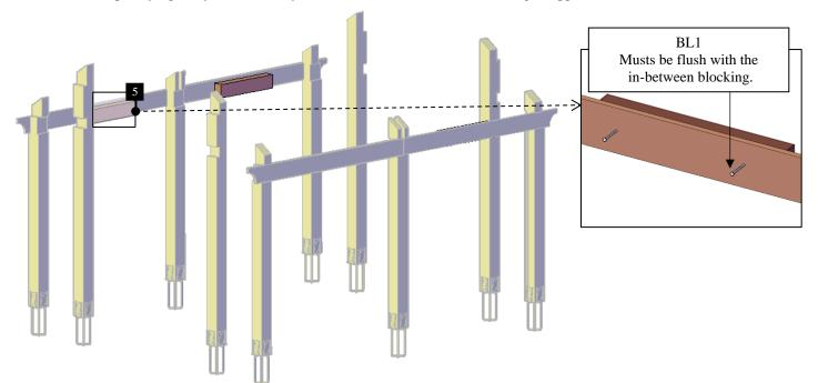
**Step 4:** Put up the interior single supports (4) into the post notches, as shown, and attach to the posts and to the in-between blocking with the previously installed bolts (tighten fully). Check the marked on each support and place as drawings shown. **Note:** Put exterior clear silicone in the support joins.
