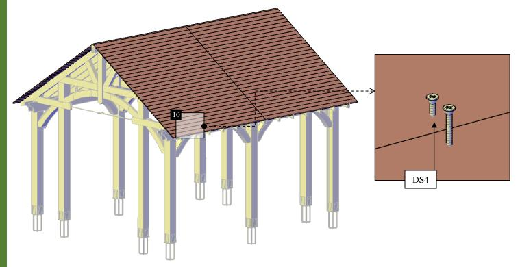
Step 26: Use 2" deck screws (DS4) to attach the roof trims (11) to the roof boards. Check the marked on each Roof trims and place as drawings shown.
