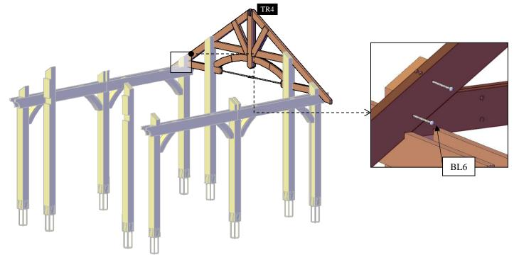
**Step 18:** Use 3/8" x 9 ¼" bolts (**BL6**) to attach the roof trusses (**1**) to the lateral posts. Check the marked on each roof truss and place as drawings shown. Note: repeat this step.
