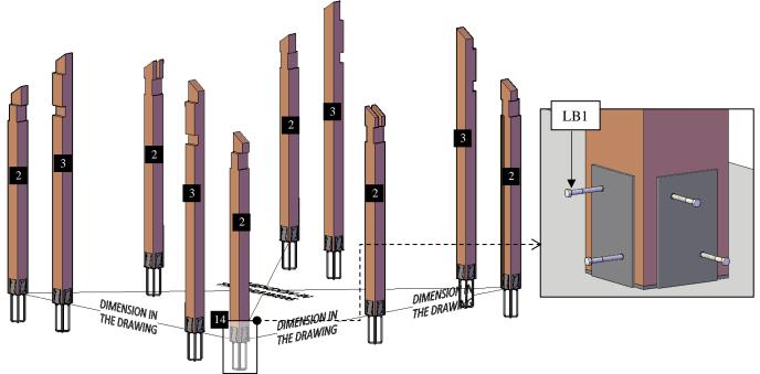
Step 2: Attach the external single supports (4) to the posts with 3/8" x 9  $\frac{1}{2}$ " bolts (BL1). Check the marked on each support and place as drawings shown.
