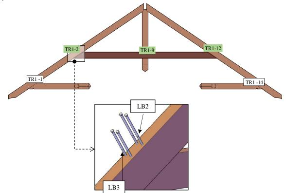
**Step 10:** Use 3/8" x 12" lag bolts (**LB2**) to attach the struts (1.5) to the rafters. Match the marked numbers in notches of the struts with the numbers in the rafters. *The marked numbers shown below corresponding at the roof trusses*.
