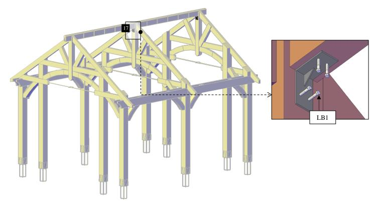
Step 22: Use 3/8" x 3 1/2" Lag Bolts (LB1) to attach the Rafter Bases (16) to the in-between blockings.
