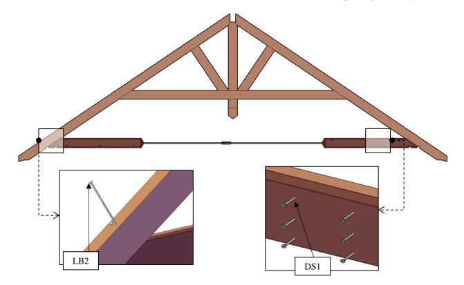
**Step 14:** Use 3/8'' x 10'' lag bolts (**LB3**) to attach the arched (**1.6**) to the hammer-beams. Match the marked numbers in the corners of the arc with the numbers in the hammer-beams. *The marked numbers shown below corresponding at the roof trusses*.
