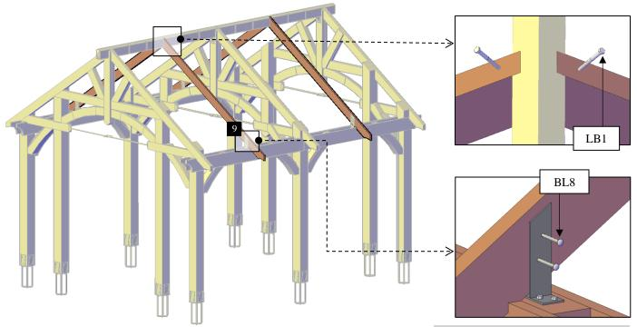
Note: The both side of the rafters must be placed at the same time (in pairs). Don't put all the rafters on one side or in the other side.
