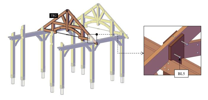
**Step 20:** Use 3/8" x 8  $\frac{1}{2}$ " bolts (**BL7**) to attach the secondary knee braces (**7**) to the perimeter roof trusses and use 3/8" x 6  $\frac{1}{2}$ " bolts (**BL5**) to the central roof trusses. After that, use 3/8" x 16  $\frac{1}{2}$ " bolts (**BL2**) to attach the secondary knee braces to the corner posts and to the central posts.
