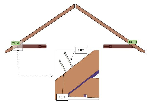
Step 8: Use 3/8" x 12" lag bolts (LB2) to attach the king post (1.3) to the rafters. Match the marked numbers in the top of the king post with the numbers in the rafters. The marked numbers shown below corresponding at the roof trusses.
