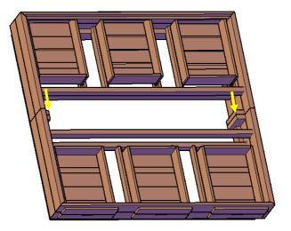
**STEP 2:** Attach the boards to the base with four screws for each board.
