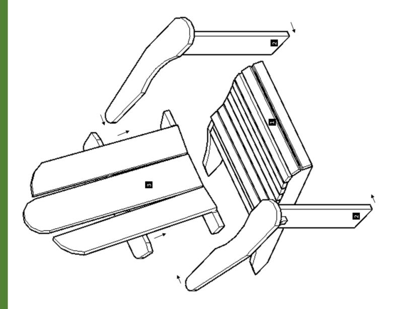
Step 1: Attach the seat (1) to the legs with arms (2) with 5/16" x 2 ½" bolts (A). Each part has a series of numbers that indicate where to attach the part with the corresponding number.
