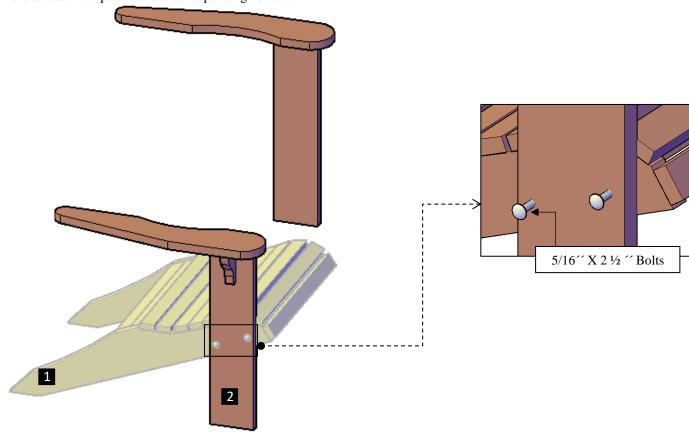
Step 2: Attach the backrest (3) to the legs with arms (2) with 5/16" x 2 1/2" bolts (A). Finally, attach the backrest (3) to the seat with 5/16" x  $2\frac{1}{2}$ " bolts (A).
