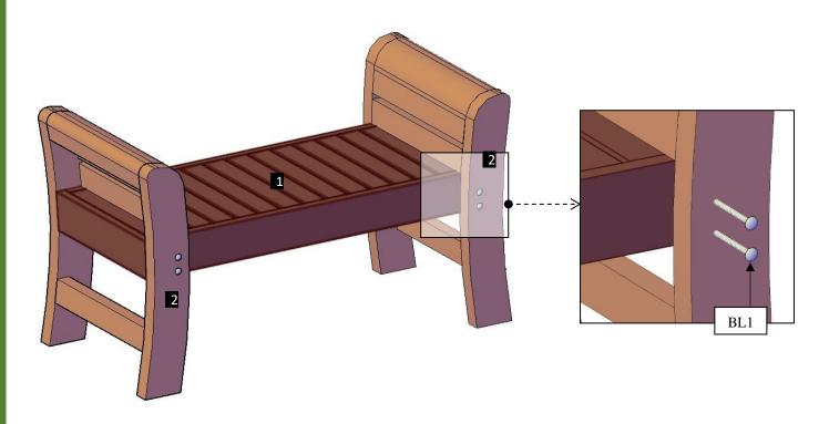
**Step 2:** Finally, attach the backrest (3) to the legs with 5/16" x 3" bolts (**BL2**), washers and nuts and to the bench seat with 5/16" x 4" bolts (**BL1**). Each part has a series of numbers that indicate where to attach the part with the corresponding number.
