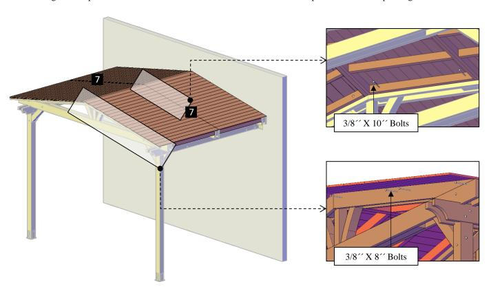
Step 13: Attach the roof panels (7) to the triangles with 6" x 1 5/8" deck screws (I).
