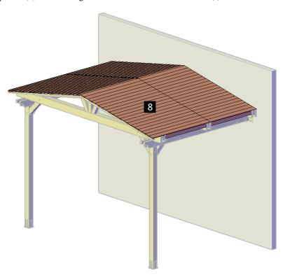
**Step 14:** Attach the roof fascia's **(8)** to the roof panels with 6'' x 1 5/8'' deck screws **(I)**. Each part has a series of numbers that indicate where to attach the part with the corresponding number.
