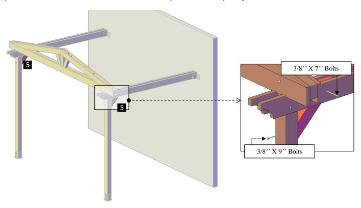
**Step 9:** Attach the secondary knee braces (6) to the triangle with 3/8" x 6 ½" bolts (**D**) and to the posts with 3/8" x 9" Bolts (**F**). Each part has a series of numbers that indicate where to attach the part with the corresponding number.
