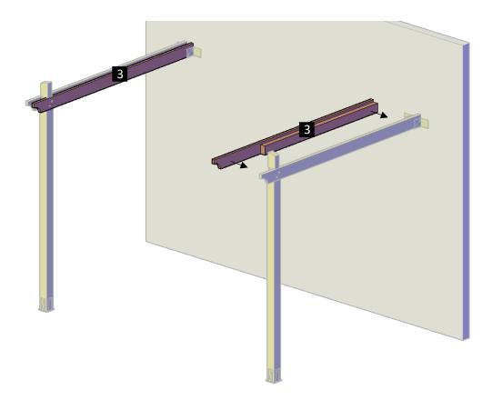
Step 5: Attach the single supports to the supports with in-between blocking, use 3/8" X 7" bolts (C).
