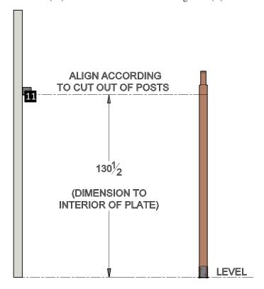
**Step 3:** Attach the single supports (2) to the posts with 3/8"x 7" bolts (C). Each part has a series of numbers that indicate where to attach the part with the corresponding number.
