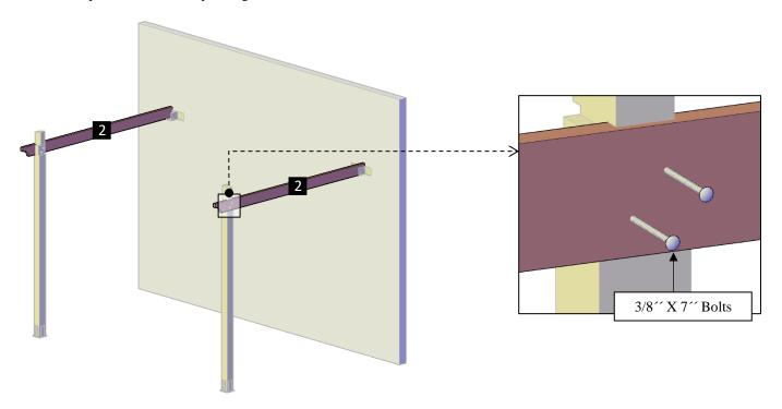
**Step 4:** Put up the supports with in-between blocking (3), into the post notches as shown and attach to the posts with the single support bolts. Each part has a series of numbers that indicate where to attach the part with the corresponding number.
