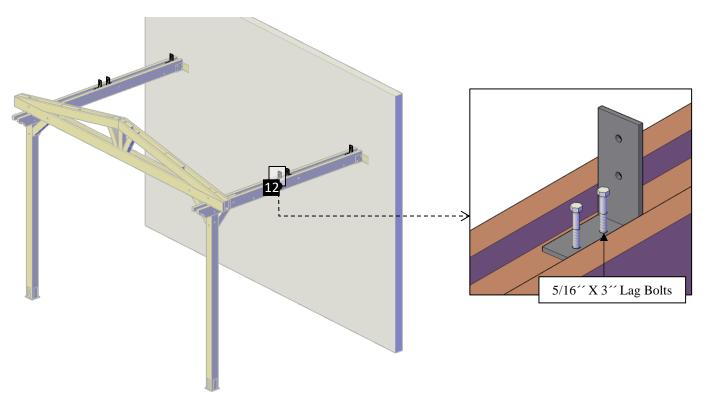
**Step 11:** Attach the central triangle (4) to the angles with 3/8" x 8" bolts (G). After that, use 5/16" x 3" lag bolts (A) to attach the back triangle (4) to the angles. Each part has a series of numbers that indicate where to attach the part with the corresponding number.
