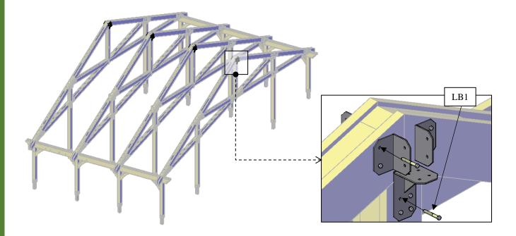
**Step 17:** Attach the ridge beam -A (8) to the L-plaques -A & B (21,22) and to the roof trusses (5) with 3/8" x 3 <sup>1</sup>/<sub>2</sub>" lag bolts (LB1). Check the marked on each ridge beam -A and place as drawings shown.
