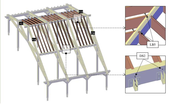
Step 21: Attach the rafter (10) to the metal plaque -F (24) and metal plaque -G (25) with 3/8" x 2 <sup>3</sup>/<sub>4</sub>" bolts (BL5). Check the marked on each rafter and place as drawings shown.
