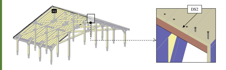
Step 26: Finally, attach the boots (15) to each post with 3" deck screws (DS1).
