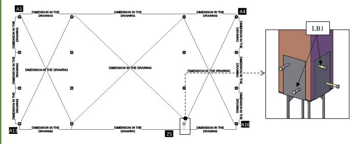
Step 2: Attach the single supports (2) to the posts with 3/8" x 9" bolts (BL1) with washer and nuts. Check the marked numbers on each support and place as drawings shown.
