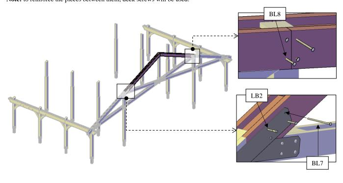
CUSTOM SCISSOR TRUSS PAVILION www.ForeverRedwood.com Step 11: Attach the section -D (5) to the king posts with 3/8" x 8 ½" bolts (BL7). After that use 3" deck screws (DS1) to attach the cover top (6) to the king post. Check the marked on each section -D and place as drawings shown. Note: return to the bolts described in the step 6 and tighten fully Note: repeat this step 3 time.
