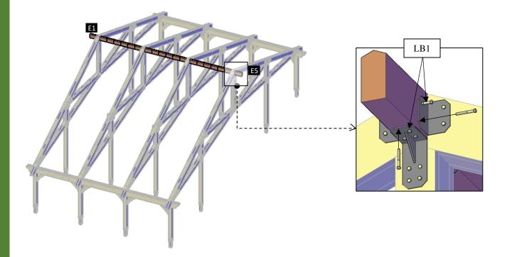
Step 18: Attach the metal plaque -E (23) to the ridge beam -B (9) with 3/8" x 4  $\frac{1}{4}$ " bolts (BL4) and 3/8" x 3  $\frac{1}{2}$ " lag bolts (LB2).
