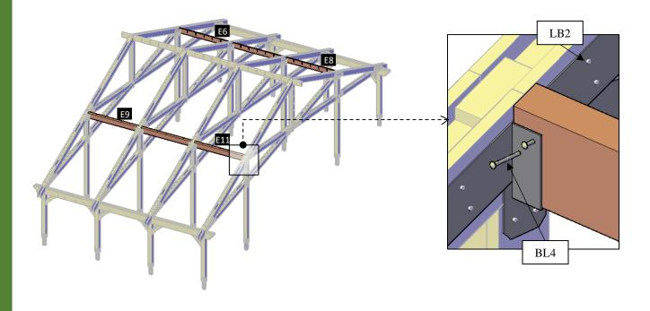
**Step 19:** Attach the metal plaque -F (24) to the supports (2) with 3/8" X 2  $\frac{1}{2}$ " lag bolts (LB3). After that use 3/8" x 2" bolts (LB4) to attach the metal plaque -G (25) to the ridge beam -B (9).
