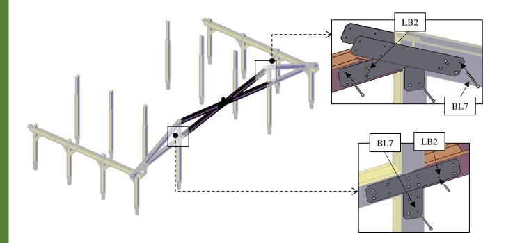
**Step 10:** Attach the section -D (5) to the posts (1) with metal plaque -D (20) use 3/8" x 8 ½" bolts (**BL7**) and 3/8" x 3 ½" lag bolts (**LB2**). After that use 3/8" x 7 ½" bolts (**BL8**) to attach the roof truss (5) to the large posts (1). Check the marked on each section -D and place as drawings shown. **Note:** drilling will be completed on site. **Note:** to reinforce the pieces between them, deck screws will be used.
