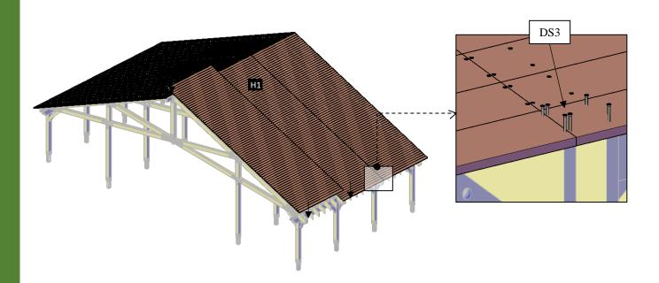
Step 24: Use 2" deck screws (DS3) to attach the fascia (13) to the roof trusses (5) and to the rafters (10). Check the marked on each fascia and place as drawings shown.
