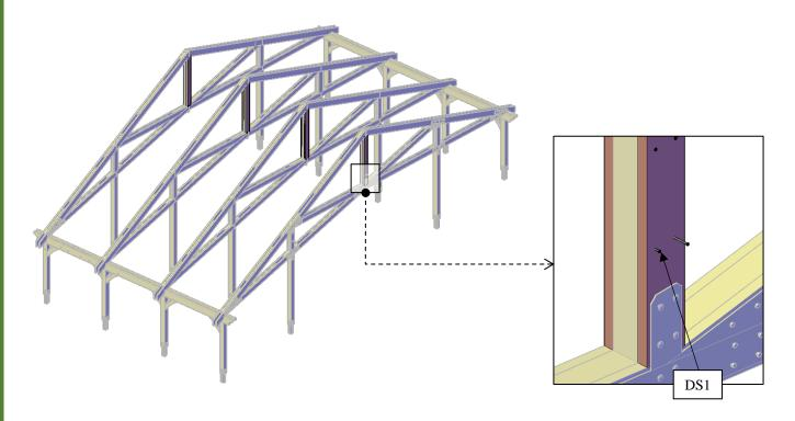
**Step 15:** Attach the secondary knee brace (7) to the roof trusses (5) with 3/8" x 9" bolts (**BL1**). After that use  $\frac{1}{2}$ " x 12" (**BL2**) to the posts (1). Check the marked on each secondary knee brace and place as drawings shown.
