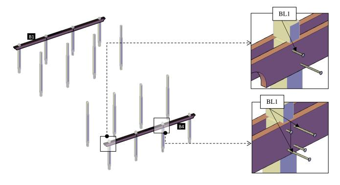
**Step 3:** Attach the in-between blocking (3) to the supports with 3/8" x 9" bolts (**BL1**) with washer and nuts. Check the marked numbers on each support with in-between blocking and place as drawings shown.
