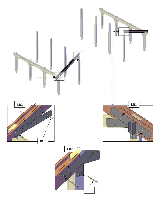
**Step 7:** Attach the section truss -B (5) to the large posts (1) with metal plaque -B & -A (18,17) and use 3/8" x 8 ½" bolts (BL7) & 3/8" x 3 ½" lag bolts (LB2). Check the marked on each section truss -B and place as drawings shown. **Note:** to reinforce the pieces between them, deck screws will be used.
