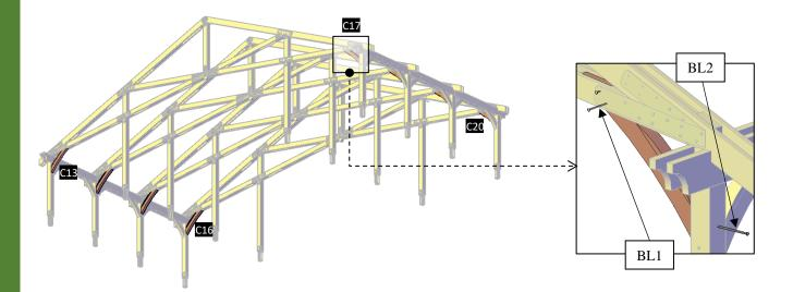
Step 16: Attach the L-plaques -A & B (21,22) and to the roof trusses (5) with 3/8" x 3 <sup>1</sup>/<sub>2</sub>" lag bolts (LB1). Check the marked on each ridge beam -A and place as drawings shown.
