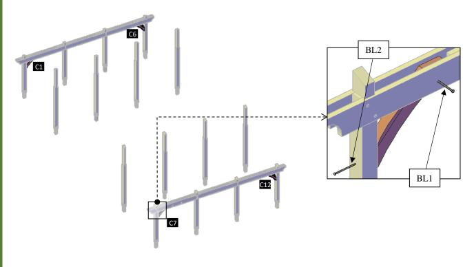
**Step 5:** Attach the central main knee braces (4) to the posts (1) with  $\frac{1}{2}$ " x 16" bolts (**BL3**). After that use 3/8" x 9" bolts (**BL1**) to the supports (2,3). Check the marked on each main knee brace and place as drawings shown.
