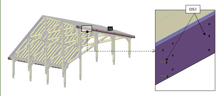
**Step 25:** Attach the overhang board (14) to the roof boards (12) whit 4" deck screws (DS2). Check the marked on each overhang board and place as drawings shown.
