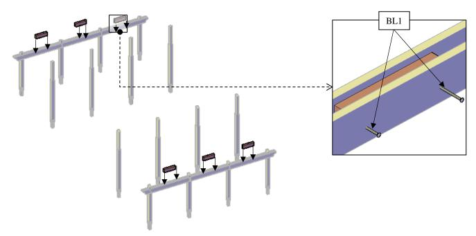
**Step 4:** Use 3/8" x 9" bolts (**BL1**) to attach the main knee brace (**4**) to the supports (**2,3**). After that use  $\frac{1}{2}$ " x 12" bolts (**BL2**) to the posts (**1**). Check the marked numbers on each main knee brace and place as drawings shown.
