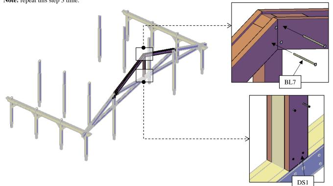
Step 12: Attach the section -C with 3/8" x 8 <sup>1</sup>/<sub>2</sub>" bolts (BL7) and metal plaque -C (19) to the king posts. Check the marked on each section -C and place as drawings shown.
