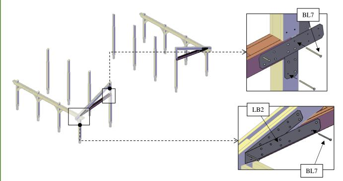
**Step 8:** Attach the section truss -C (5) between them with metal plaque -C (19) and 3/8" x 8 ½" bolts (**BL7**) & 3/8" x 3 ½" lag bolts (**LB2**). Check the marked on each section truss -C and place as drawings shown.
