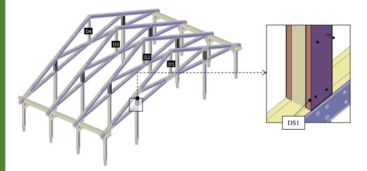
Step 14: Attach the cover top (6) to the king posts with 3" deck screws (DS1). Check the marked on each cover top and place as drawings shown.
