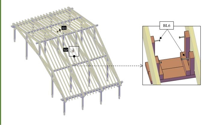
Step 23: Attach the roof board (12) to the rafters (10) and to the roof trusses (5) with 2" deck screws (DS3). Check the marked numbers on each roof board and place as drawings show.
