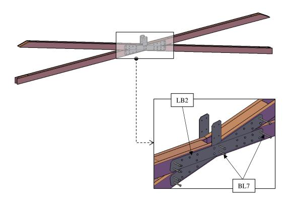
**Step 9:** Attach the section truss -D (5) to the posts (1) with metal plaque -B & -D (18,20) use 3/8" x  $8\frac{1}{2}$ " bolts (**BL7**) and 3/8" x  $3\frac{1}{2}$ " lag bolts (**LB2**). Check the marked on each section truss -D and place as drawings shown
