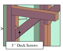
Step 6: Attach the shelves supports (6) to the wall panels with 3<sup>''</sup> deck screws (C). Each part has a series of numbers that indicate where to attach the part with the corresponding number.
