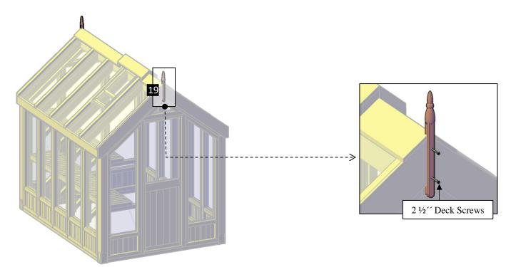
Step 22: Finally, attach the boots (20) to the posts with  $2^{\prime\prime}$  deck screws (D). Each part has a series of numbers that indicate where to attach the part with the corresponding number.
