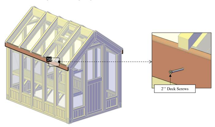
Step 19: Attach the front and back fascia boards (17) to the wall panels with  $2^{\prime\prime}$  deck screws (D). Each part has a series of numbers that indicate where to attach the part with the corresponding number.
