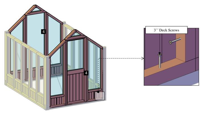
**Step 5:** Attach the small and large braces (5) to the wall panels with  $3^{\prime\prime}$  deck screws (C). Attach with  $3^{\prime\prime}$  deck screws (C) in the acrylic direction and the wall panel direction, as shown below. Each part has a series of numbers that indicate where to attach the part with the corresponding number.
