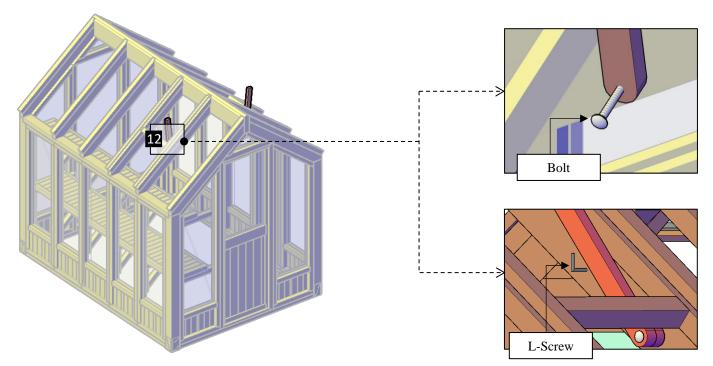
Step 14: Use 3" deck screws (C) to attach the polycarbonate (13) and the cover trims (14) to the rafters. Each part has a series of numbers that indicate where to attach the part with the corresponding number.
