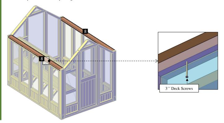
**Step 9:** Attach the perimeter rafters (9) to the supports with 6'' deck screws (**F**) and to the wall panels with 3'' deck screws (**C**) . Each part has a series of numbers that indicate where to attach the part with the corresponding number.
