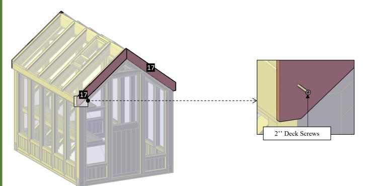
**Step 20:** Attach the top fascia boards (18) to the rafters with  $2^{\prime\prime}$  deck screws (**D**). Each part has a series of numbers that indicate where to attach the part with the corresponding number.
