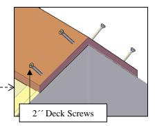
**Step 21:** Attach hip-knob (19) to the front and back fasci boards with  $2\frac{1}{2}$  deck screws (E). Each part has a series of numbers that indicate where to attach the part with the corresponding number.
