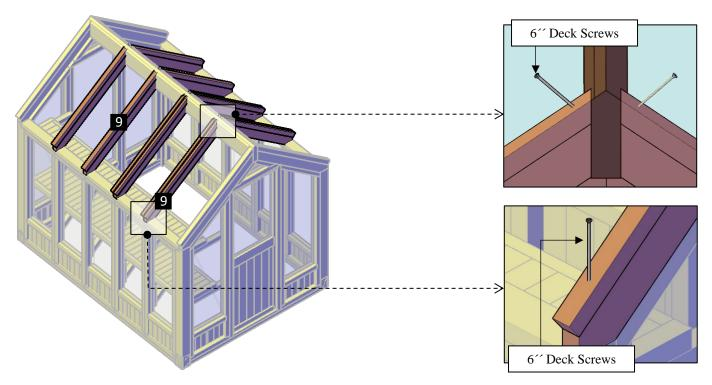
**Step 12:** Use 3<sup>--</sup> deck screws (**C**) to attach the window supports (**11**) to the rafters. Each part has a series of numbers that indicate where to attach the part with the corresponding number.
