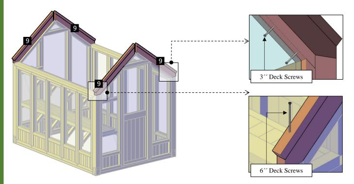
Step 10: Place the ridge beam (10) between the rafters (9). After that, use  $6^{\prime\prime}$  deck screws (F) to attach the rafters to the ridge beam (9). Each part has a series of numbers that indicate where to attach the part with the corresponding number.
