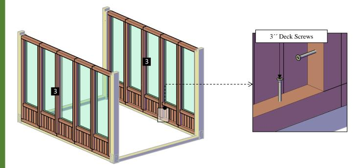
**Step 4:** Attach the wall panels (4) to the bottom wall frame with 3<sup>''</sup> deck screws (C). Then, use 3<sup>''</sup> deck screws (C) to attach the wall panels together and to the posts. Each part has a series of numbers that indicate where to attach the part with the corresponding number.
