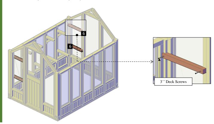
**Step 7:** Attach the small and large shelves (7) to the braces and to the shelves supports (6) with 3<sup>---</sup> deck screws (C). Attach from the bottom in the front side and from the top in the back side. Each part has a series of numbers that indicate where to attach the part with the corresponding number.
