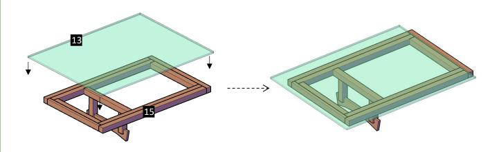
Step 16: Attach the windows (15) to the rafter with 3<sup>''</sup> deck screws (C). Each part has a series of numbers that indicate where to attach the part with the corresponding number
