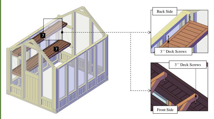
Step 8: Attach the supports (8) to the wall panel with 3" deck screws (C). Each part has a series of numbers that indicate where to attach the part with the corresponding number.
