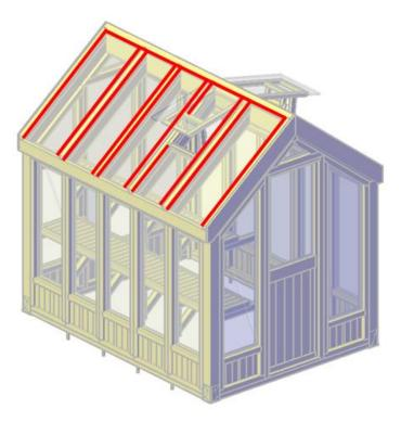
**Step 18:** Attach the lateral fascia boards (16) to the wall panels with  $2^{\prime\prime}$  deck screws (D). Each part has a series of numbers that indicate where to attach the part with the corresponding number.
