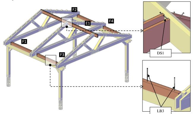
**Step 14:** Attach the rafter (10) to the ridge beam (8) with 4" deck screws (**DS2**) and to the support rafters (9) with 3" deck screws (**DS1**). Check the marked numbers on each rafter and place as drawings shown.
