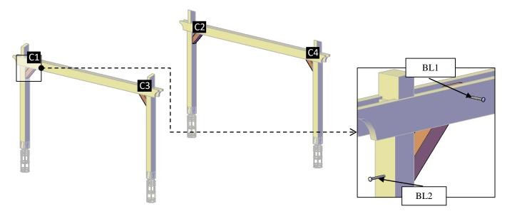
Step 6: Attach the top in-between blocking (5) to the supports in-between blocking (2,3) with 3" deck screws (DS1). Check the marked numbers on each top and place as drawings shown
