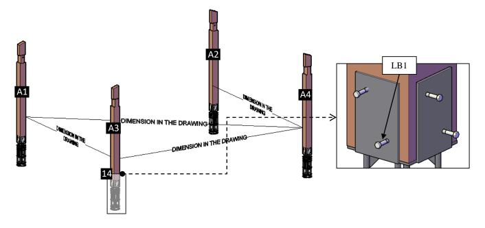
**Step 2:** Attach the single supports (2) to the posts (1) with 3/8" x 8" bolts (**BL1**). Check the marked numbers on each single support and place as drawings shown.
