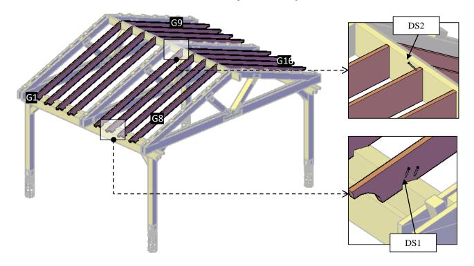
Step 15: Attach the secondary rafter (11) to the purlins (12) with 3" bolts (DS1). Check the marked numbers on each purlin and place as drawings shown.
