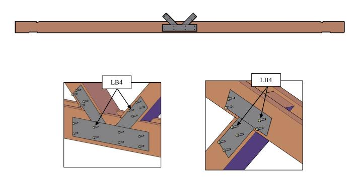
Step 8: Attach the Plaques in the Flower (16) to the central tie beam (6.1) with 3/8" x 1 ½" lag bolts (LB4) and to the struts (6.2).
