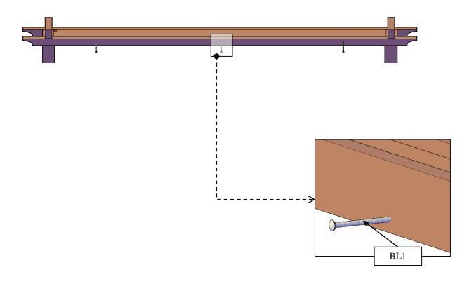
**Step 5:** Attach the main knee braces (4) to the supports (2,3) with 3/8" x 8" bolts (**BL1**) and to the posts (1) with 3/8" x 12" bolts (**BL2**). Check the marked numbers on each main knee brace and place as drawings shown.
