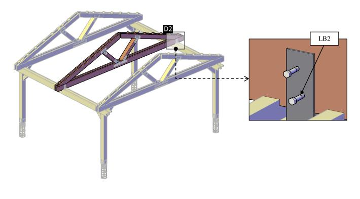
**Step 13:** Use 3" deck screws (**DS1**) to attach the ridge beam (**8**) to the roof trusses (**6**). After that use 3/8" x 12" lag bolts (LB3) to attach support rafter (**9**) to the support in-between blocking (**3**). Check the marked numbers on each ridge beam and place as drawings shown.
