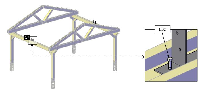
**Step 12:** Use 3/8" x 3" lag bolts (**LB2**) to attach the roof truss (6) to the metal plaques -B (17). Check the marked numbers on each roof truss and place as drawings shown.
