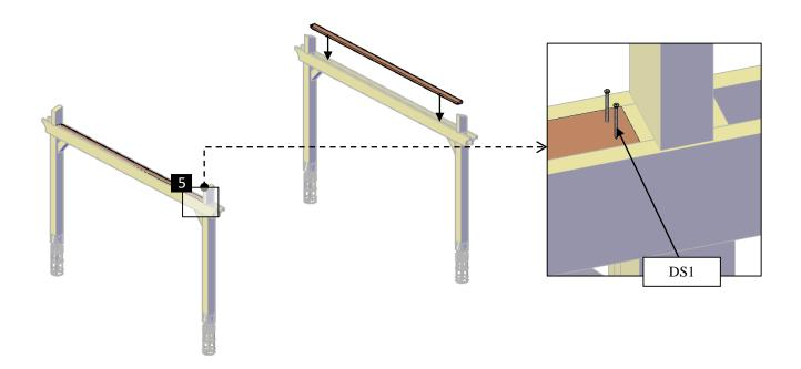
Step 7: Attach the Plaques in the Flower (16) to the lateral tie beams (6.1) with 3/8" x 1 ½" lag bolts (LB4) and to the struts (6.2).
