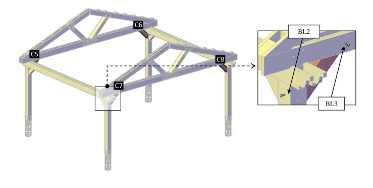
**Step 11:** Use 3/8" x 3" lag bolts (**LB2**) to attach the metal plaque -B (**17**) to the support in-between blocking (**3**). Check the marked numbers on each metal plaque -B and place as drawings shown.
