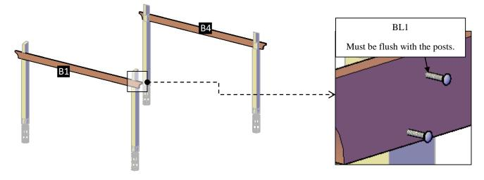
**Step 3:** Place the supports with support in between blocking (3) into the post notches. After that, return to the bolts described in the step 2 and tighten fully. Check the marked numbers on each support with in-between blocking and place as drawings shown. *Note: put silicone in joints of the supports with in-between blocking.*
