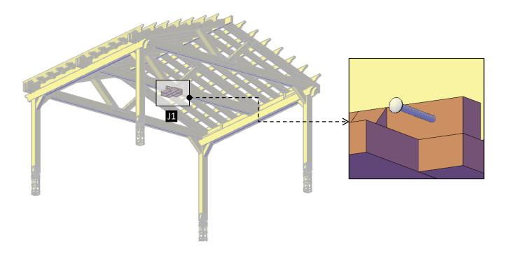
Step 17: Finally, Attach the boot (14) to the posts (1) with 3" deck screws (DS1). Check the marked numbers on each boot and place as drawings shown.
