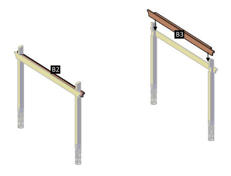
Step 4: Attach the single supports (2) to the supports with in-between blocking (3), use 3/8" x 8" bolts (BL1).
