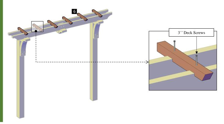
**Step 7:** Attach the boots (6) to the posts with 3<sup>---</sup> deck screws (F). Each part has a series of numbers that indicate where to attach the part with the corresponding number.
