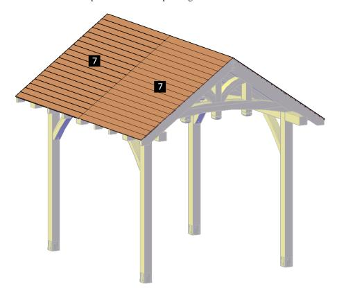
Step 9: Attach the boots (8) to the posts with 8" x 3" deck screws (I).
