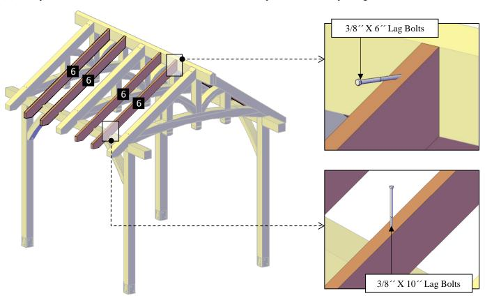
**Step 7:** Attach the perimeter rafters (6) to the supports with 3/8" x 10" lag bolts (E) and to the roof beam with 5/16" x 4" lag bolts (G). Each part has a series of numbers that indicate where to attach the part with the corresponding number.
