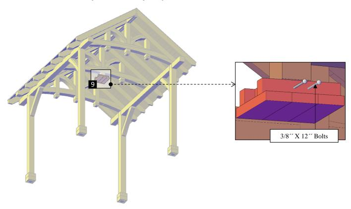
**Step 11:** Attach the perimeter ceiling fan bases (9) to the rafters with 5/16 'x  $4\frac{1}{2}$ ' bolts (**K**). Each part has a series of numbers that indicate where to attach the part with the corresponding number.
