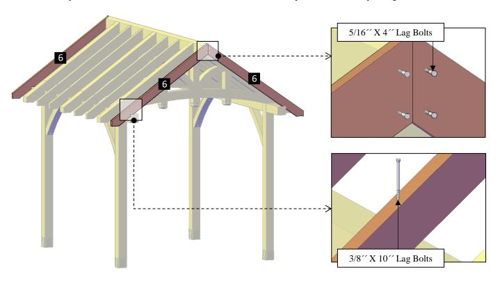
**Step 8:** Use 6" x 2" deck screws **(H)** to attach the roof boards **(7)** to the rafters and to the triangles. Each part has a series of numbers that indicate where to attach the part with the corresponding number.
