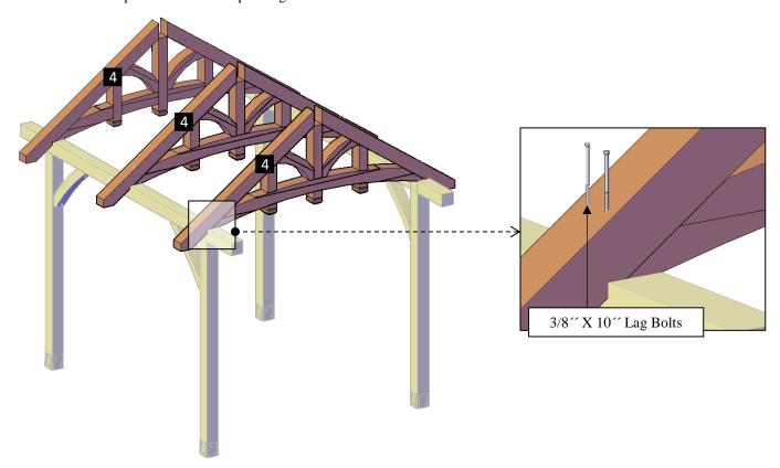
**Step 5:** Place the roof beam (5), into the triangle notches as shown. After that, use 3/8 x 6 lag bolts (F) to attach the triangles to the roof beam. Each part has a series of numbers that indicate where to attach the part with the corresponding number.
