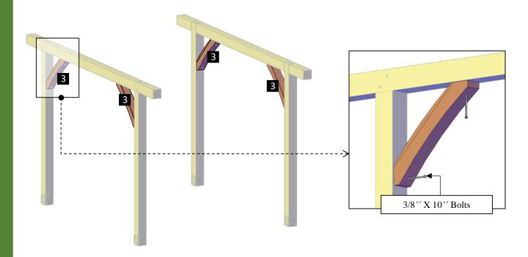
**Step 4:** Attach the triangles (4) to the supports with 3/8" x 10" lag bolts (E). Each part has a series of numbers that indicate where to attach the part with the corresponding number
